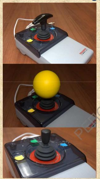
A computer joystick combines the functions of a mouse and joystick. To control the cursor is a handle with three buttons. The buttons on the right and left correspond to the right and left buttons of the normal mouse. Using the top button, you can select text or an object.
