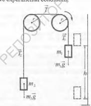
Thus, for the traditional Atwood machine, in the presence of two cargoes conected by a weightless thread and two blocks rotating with friction, the basic system of equations, taking into account the possibility of detecting the acceleration of translational motion through electronic fixation of the time for the passage of arbitrarily varied masses of cargo through a variable height, is
